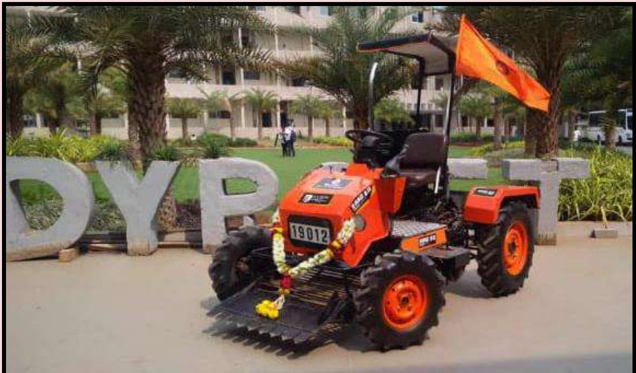
Self Propelled onion harvester developed by Team DYP CET
