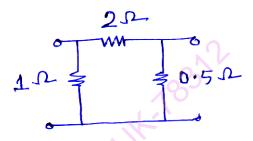
c) Find short circuit admittance parameters for the given circuit.
