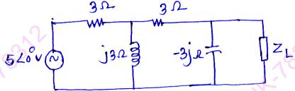
d) Verify reciprocity theorem with the source and an ammeter for following network.
