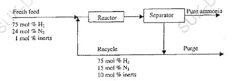
The single pass conversion for H<sub>2</sub> in the reactor is 20%. Calculate amount of H<sub>2</sub> lost in the purge as a percentage of H<sub>2</sub> in fresh feed. [8]
